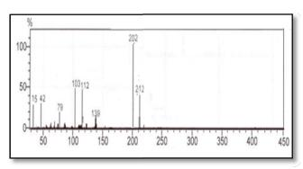
Fig. 5: Mass Spectra of compound B2
